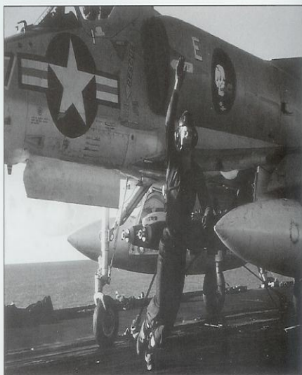
Signalling all is ready, a crewman gets out of the way before a VA-12 A-4C launches from 'FDR' on 6 September 1966. The 'Charlie' carries two 300-gallon fuel tanks and all its bombs on the centreline multiple ejection racks. Note the striking 'Kiss of Death' squadron insignia on the fuselage (Neal Crowe)
